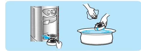
1. When Red Overflow Indicator is visible, Drip Tray must be emptied and cleaned-up
